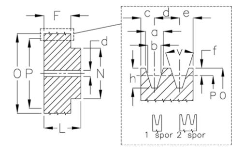
$\begin{array}{lll} d & = 10 \\ F & = 25 \\ L & = 45 \\ N & = 50 \\ Number of ribs = 1 \\ O & = 97.0 \\ P & = 90 \\ Type & = B \end{array}$
